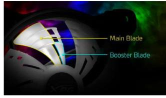
Innovative dual-layer fan blade design is comprised of the Main Blade and the Booster Blade. Both function simultaneously to enhance airflow and static pressure, while minimizing wind resistance hence less noise during operation.
