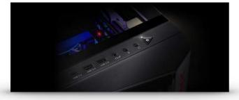
A versatile combo of I/O ports, including USB Type-C and Type-A, make life easy. Also, a unique power on/off button that's shaped like a play button launches you into battle.
