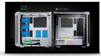
The XPG BATTLECRUISER accommodates different storage configurations, up to three 3.5" or six 2.5" HDDs/SSDs.
