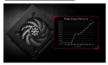
XPG CYBERCORE is the latest XPG and Nidec collaboration, utilizing our highest tier XPG VENTO PRO 120 PWM Fan for its high cooling efficiency, featuring Dual Bearing and patented technology to maintain an excellent balance between noise and life expectancy (60,000 hours at 60°C).
